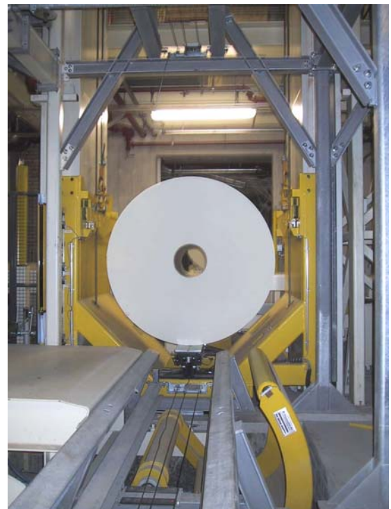
ACTIV System- Vertical Transfer Lift & Conveyor Interface
