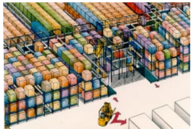
Trailer Load Staging—forklift pulls loads from staging slot face and positions them directly onto their assigned trailer.
