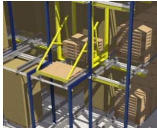
P-CAT accumulates standard and custom captive pallets and delivers them to an ACTIV input point for reuse
