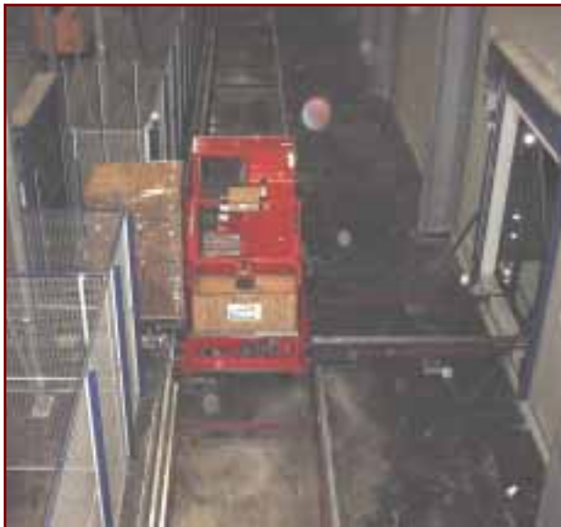
ACCESS Vehicle Picking up a Pallet at the Entry Way to the ACCESS System
