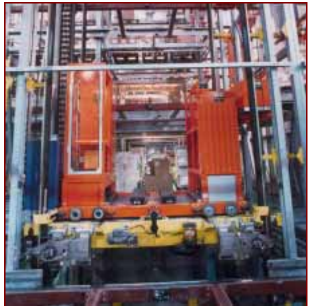
ACCESS Vehicle on Lift with Battery Change-out Stations
